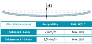
\* Square shapes could increase the overall bow tolerance
