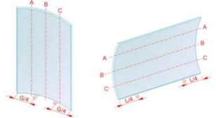
It will be horizontally placed a straightedge ruler with 0,1 mm intervals along the length of the glass to measure the gap between the glass specimen and the ruler.
