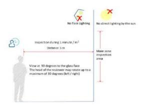
If a revision under reflection conditions is required (from outside), the glass units shall be observed in the same way they would be observed once they are installed on façade.
